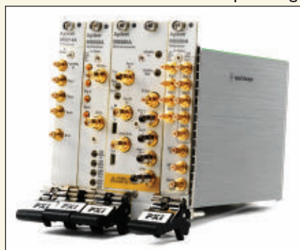
▲ Fig. 1 M9393A PXIe performance vector signal analyzer.
